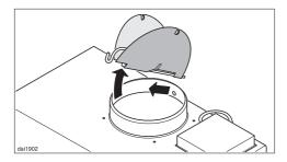
Remove the non-return flap from the exhaust connection.
