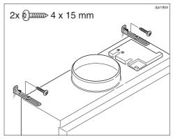
■ Attach the retaining bracket to the rear panel.
