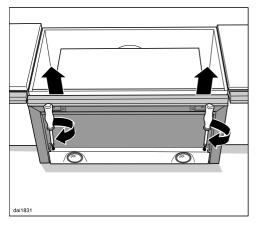
Use a screwdriver to align the fume deflector correctly.
