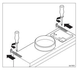
Loosen the retaining bracket screws and push the brackets back against the rear wall.
