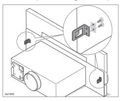
When installing a 31 <sup>1</sup>/<sub>2</sub>" or 35 <sup>7</sup>/<sub>16</sub>" (80 or 90 cm) wide hood in a 23 <sup>5</sup>/<sub>8</sub>" (60 cm) wide wall unit while the fume deflector is pulled out, unscrew the two fume deflector spring mounts.
