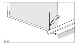
Draw a vertical line up both inside walls of the cabinetry from the front of the spacer strip.
