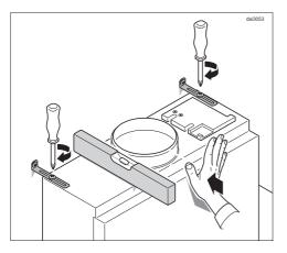
Align the casing and screw the retaining bracket onto the casing.
