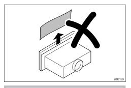
To avoid scratching the fume deflector, do not remove the protective film between the fume deflector and the casing until the hood has been placed in the cabinetry
